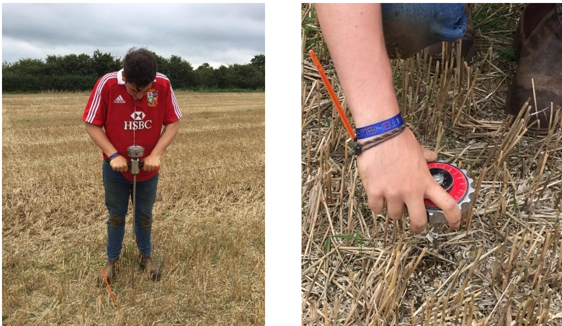
Figure 10. Measurement of soil penetration resistance (left) and shear strength (right)
