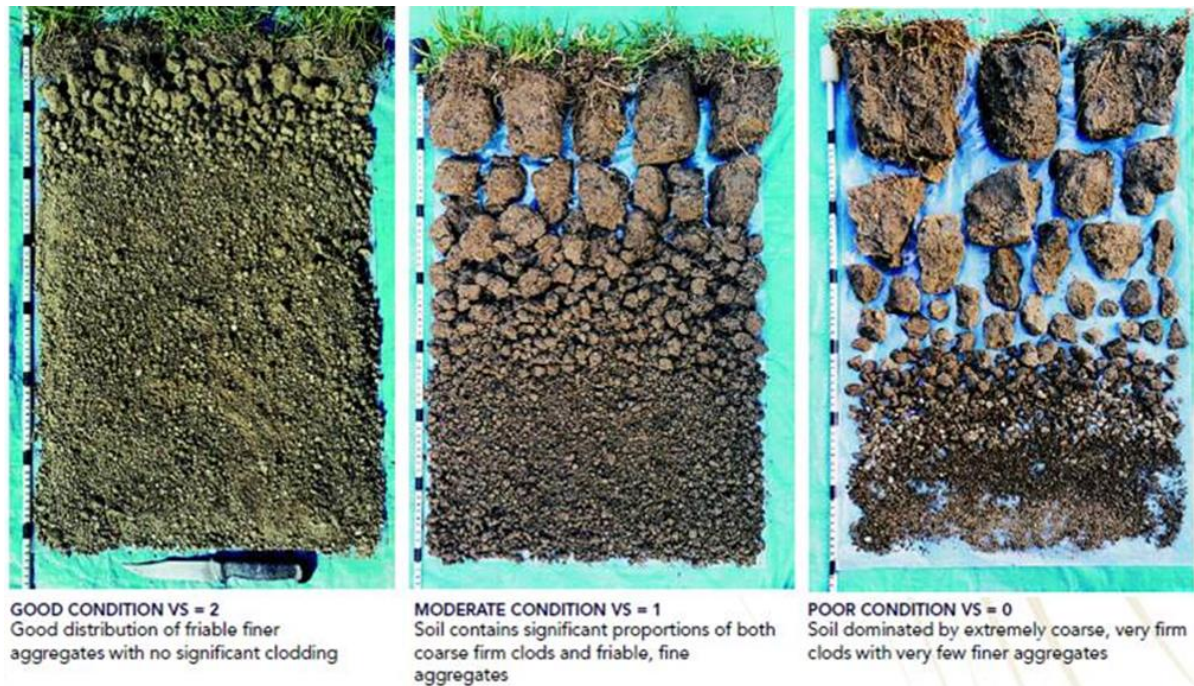
Figure 11. VSA method for visual scoring of soil structure and consistence
